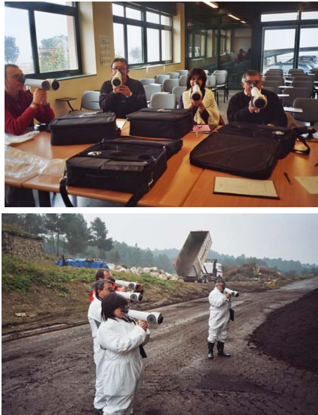
Figure 3. Training (above) and field intercomparison (below) with the Nasal Ranger™ at the source-separated MSW composting facility
